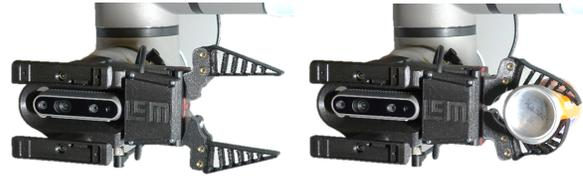
Fig. 7. Elastic fingers with fin ray design in opened and closed configuration. (The LED lights still need to be installed next to the Realsense camera.)
