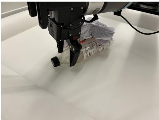
Fig. 12. Gripping in the center of the bounding box of the (visible) contour of the bottle.
