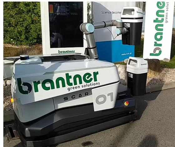
Fig. 1. SCARAB during operation while changing the container.
