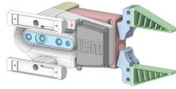
Fig. 6. Different designs of the gripper: Left with rigid fingers, right with fin ray design. In the right figure, the Gimatic gripper is shown in red and blue and the capacitor box is under the lid with the LCM logo.
