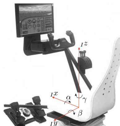
Fig. 1: Motion simulator mounted on the parallel platform
