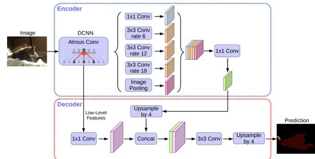
Fig. 2: The architecture of the Deeplabv3+ [1].
