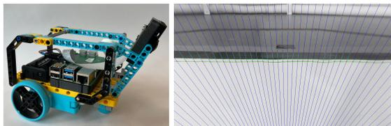
Fig. 1: The assembled robot used for the evaluation of this paper. Fig. 2: Generating laser range data for localization using low-cost camera images.
