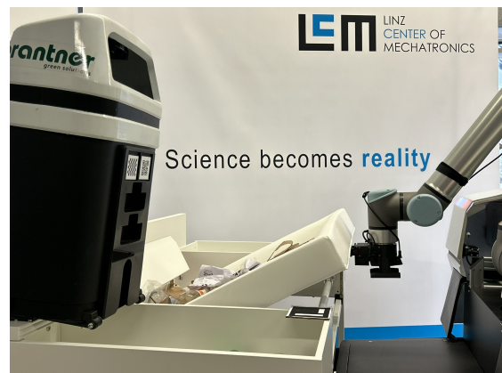
Fig. 5. The sorting table is also operated by the robotic arm without additional actuators.
