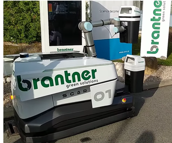
Fig. 1. SCARAB during operation while changing the container.
