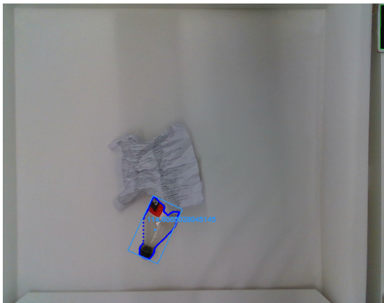
Fig. 11. Computation of the gripping point: bounding box (light blue rectangular) with center point and its rotation in degree.
